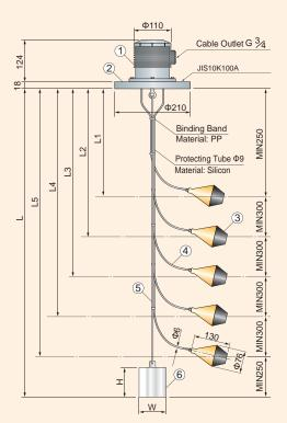
\*Product below minimum in distance between floats can be available. (Prior arrangement is necessary.)
