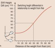
Curbing line:Switching Height Differential Subject to the weight position
